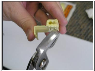
Using a pliers remove the steel insert in the middle of the connector. It just slides out.
