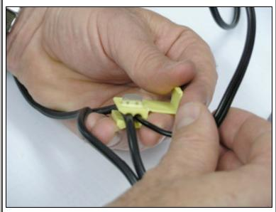
Put the metal blade back into the slot on the yellow connector
