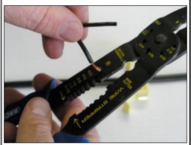
For installation cut off any unshielded wire from your fixture. An exposed copper end is not required when using this connector.
