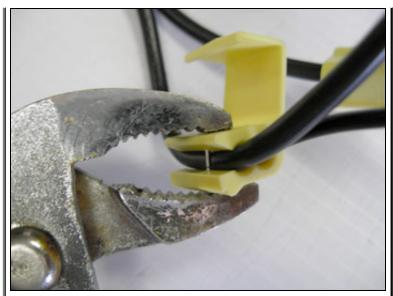
The blade will make contact with both wires for a secure connection
