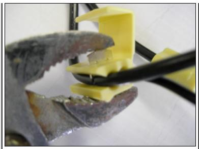
Gently push the metal blade into the wires with pliers.
