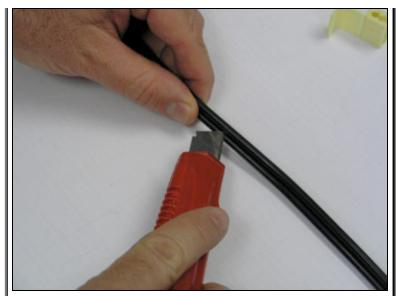
Carefully cut the center of the main feed wire so you can separate the two conductors. Use a razor knife in the very center of the wire, running parallel.
