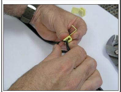
The feed wire should easily enter and exit the connector from both sides
