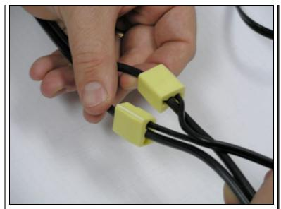
Use one connector on each side of the feed wire to complete the connection. Place your wiring under the ground cover in your garden. There is no need to bury the wiring in the ground. This way the wire will stay somewhat dry and be easy to service.
