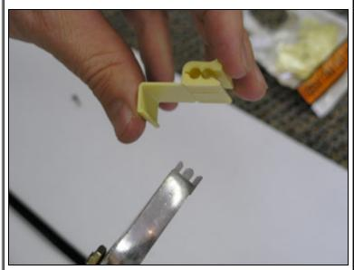
Once the steel connector is removed the wire is ready to insert.
